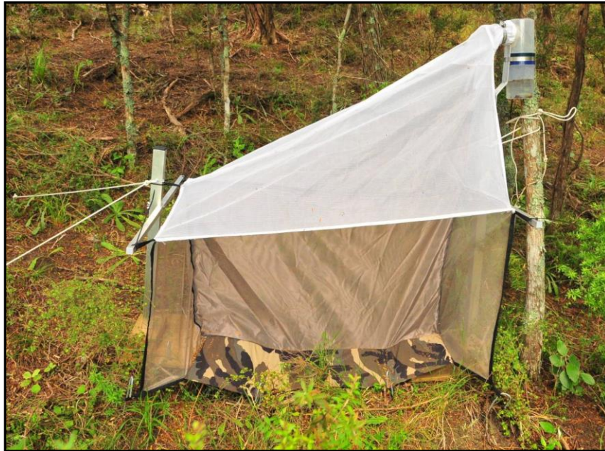
Figure 3 A malaise trap used to collect flying insects, particularly flies, wasps and beetles.
